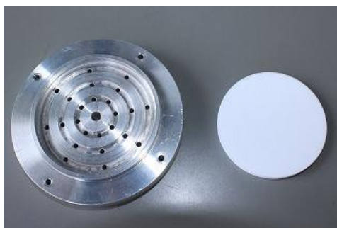
(a) Fixture plate (b) Porous polyethylene resin Fig.1 Component of porous vacuum chuck
